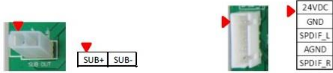
J1: Subwoofer Output Connector
