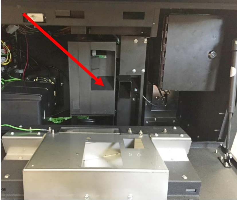
Figure 12: Hopper Position in the Machine
