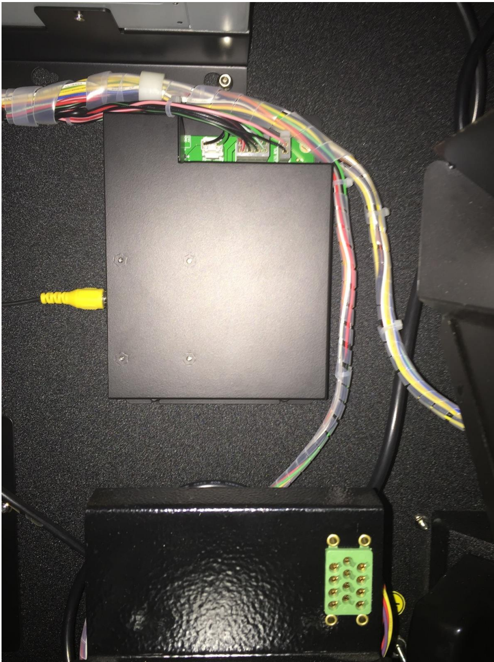
Figure 28: Audio Amplifier Position in the Machine
