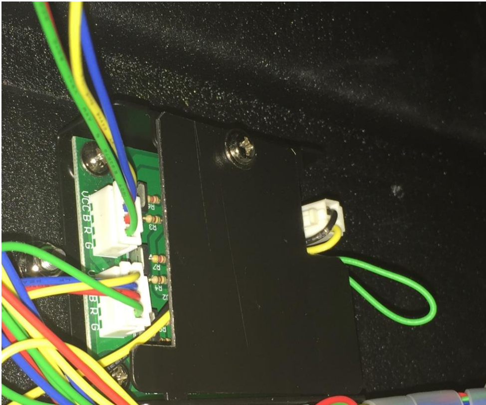
Figure 31: LED Control Board Position in the Machine
