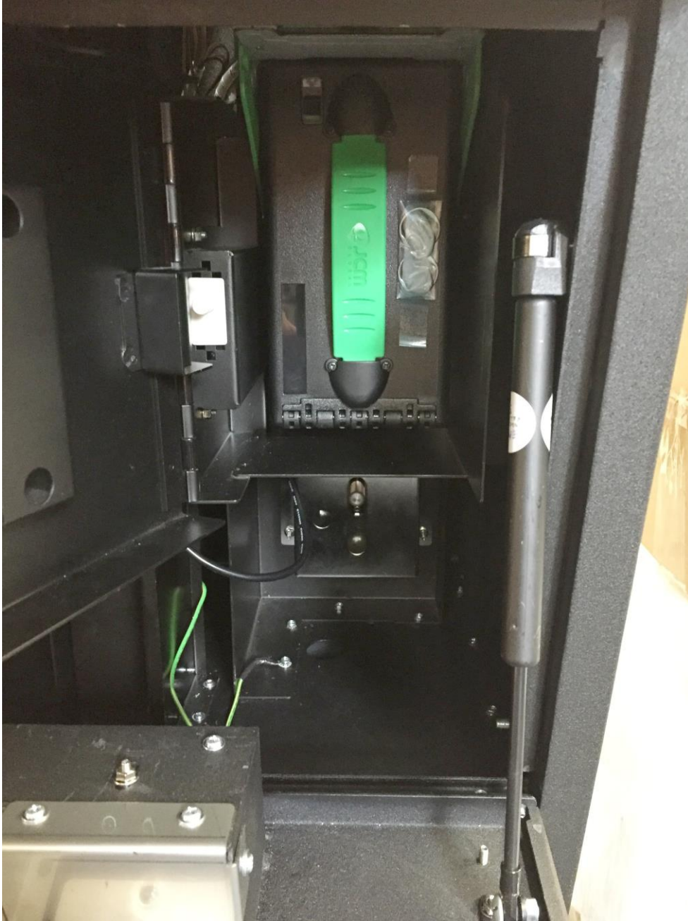
Figure 15: Bill Acceptor Position in the Machine
