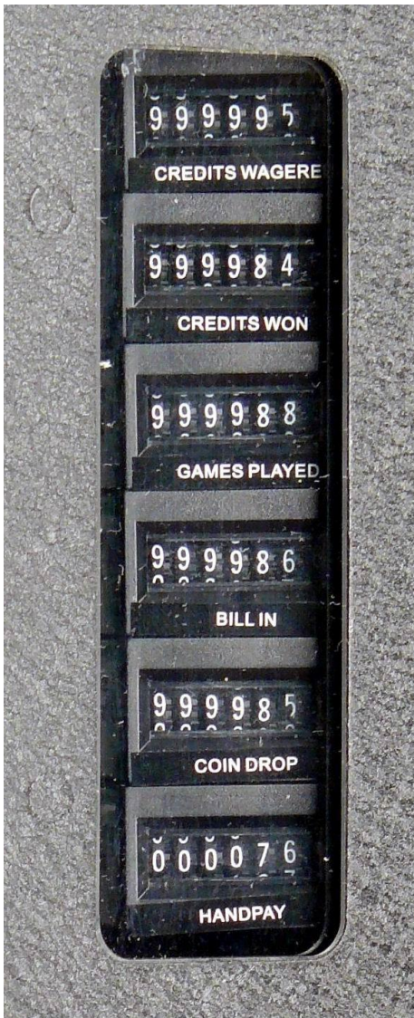
Figure 24: Hardware Meters Position in the Machine
